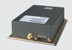
The XPRO is designed for long operating periods without maintenance (long-life rubidium lamp and extended crystal control range). With a  $5.0 \times 10^{-11}$  per month aging, the oscillator will maintain  $1.0 \times 10^{-9}$  frequency accuracy for 10 years or longer without recalibration.
